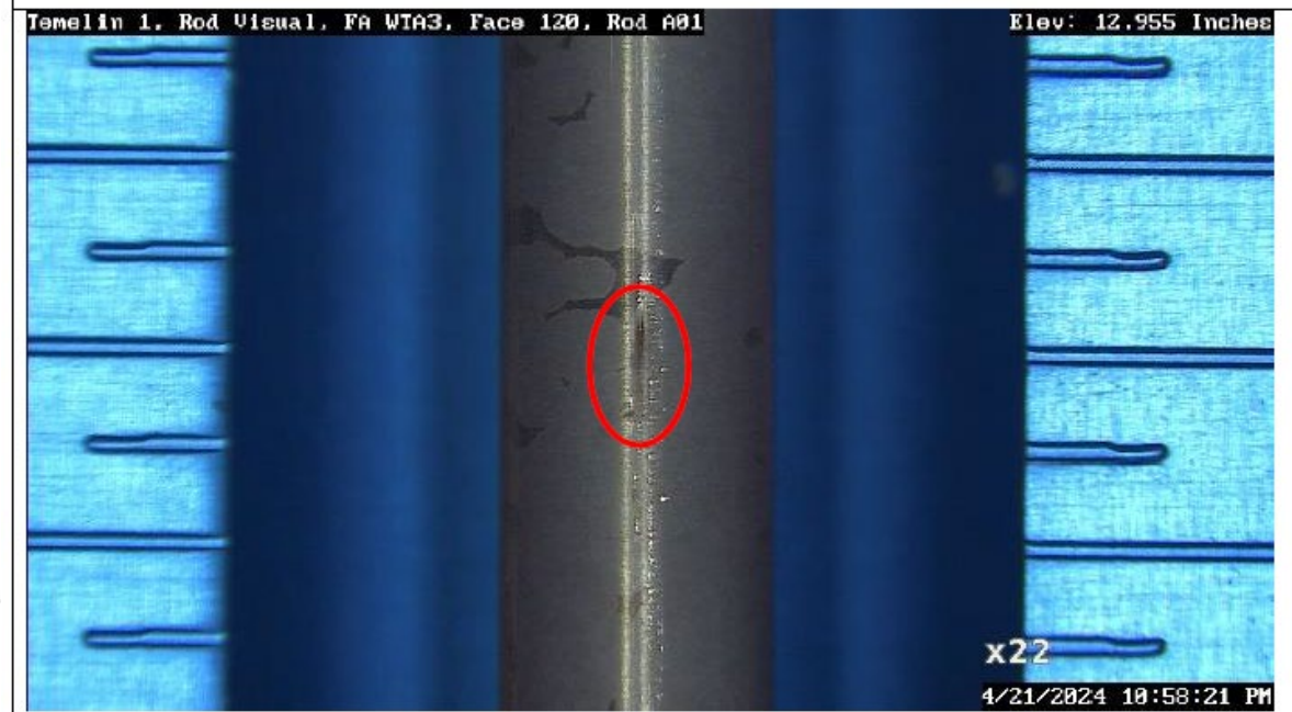
Typical contact marks on rod A01
