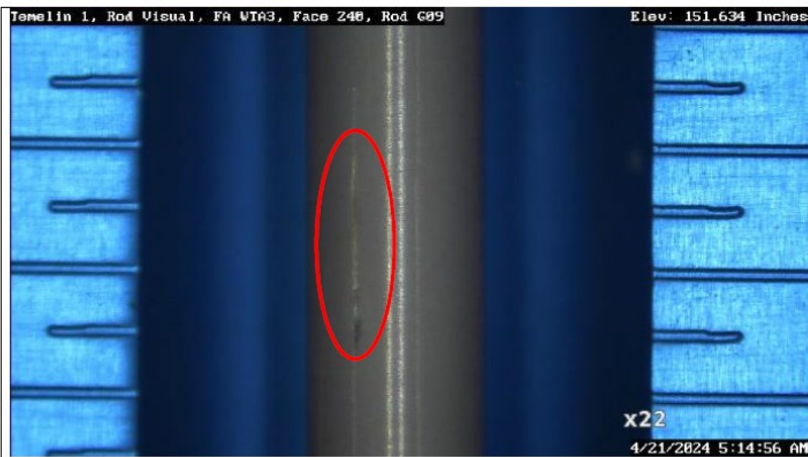
Contact mark and scratch from rod extraction, rod G09
