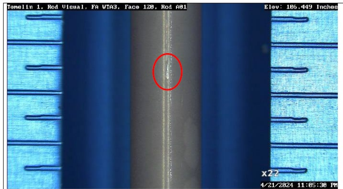
Typical contact marks on rod A01
