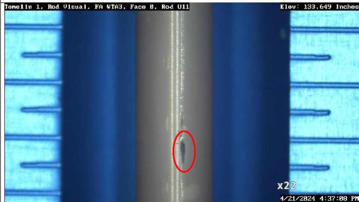
Contact mark on rod U11
